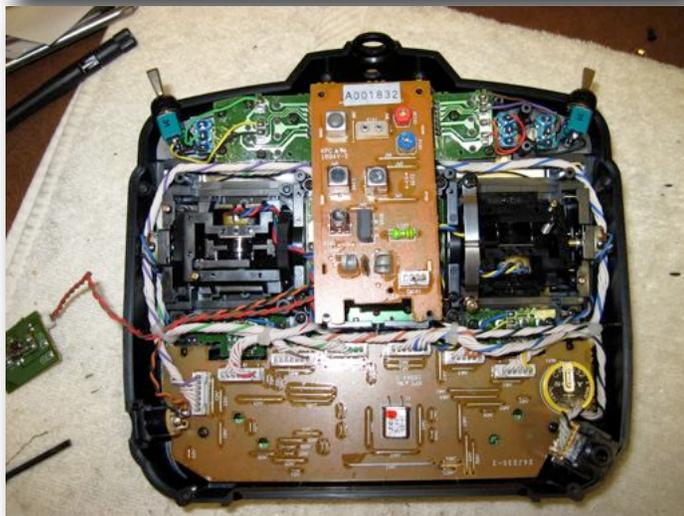
the 2.4 GHz spread spectrum with the components that are available from FrSky. The radio didn't have a plug-in RF module but inside the transmitter's case, the RF circuitry was segregated nicely onto a board that could be unplugged, removed to facilitate connection of a FrSky 2.4 GHz RF board of similar
